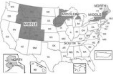
DESIGN ROOF LOAD ZONE MAP: MIDDLE 30 PSF
